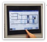
Optional, remotely located, user interface panel is available when increased accessibility is important.
