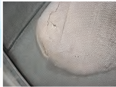
Overheated Rotor Appearance
