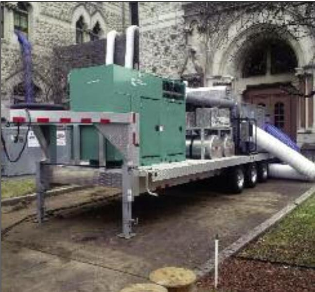
Trailer-mounted - MS-6000/5000 with heat recovery.
