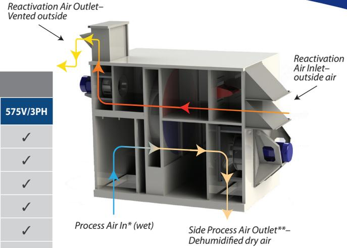
\* Supply air in can be positioned on bottom, side, top, or end air inlets
